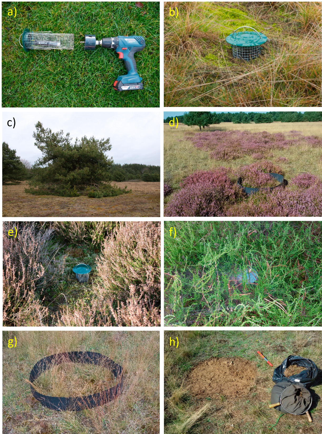
Fig. 2. Photographs taken at the nature reserve Marienfließ (MF) in 2021. (a) Cordless electric drill with circular saw attachment, for drilling holes into the frozen ground into which cylindrical wire bird feeders were placed with the sensors of the data loggers suspended inside. (b) Data logger placed in an open area between solitary pine trees (MF_3). (c) Single standing pine with branches almost resting on the ground (MF_2). (d) Open area of heath with sparse stands of Calluna . The enclosed area is 1 m 2 and is the area from which all the vegetation was harvested (biomass). (e) Data logger in a stand of Calluna . (f) Over the course of the growing season the data logger was completely overgrown (MF_4). (g) Enclosed open area with Deschampsia flexuosa (L.) Trin. and Festuca ovina agg. L. prior to harvest of vegetation (MF_5). (h) Same site after vegetation is collected (biomass) and the litter including the epigeic rove beetles is sieved through a conventional 8 mm sieve.
